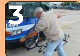
To unload, release support arm and lift bike from the rack. Return rack to the upright position.
