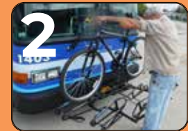
Place bike wheels into slots labeled "front" and "rear." Pull out bike support and lift it over front wheel. The Summer in the arm will keep your bike secure while the bus is moving.
