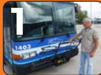
1 Pull up on release and lower rack.
