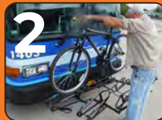
2 Place bike wheels into slots labeled "front" and "rear." Pull out bike support and lift it over front wheel. The Summer in the arm will keep your bike secure while the bus is moving.
