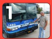
Pull up on release and lower rack.
