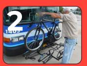
Place bike wheels into slots labeled "front" and "rear." Pull out bike support and lift it over front wheel. The Summer in the arm will keep your bike secure while the bus is moving.
