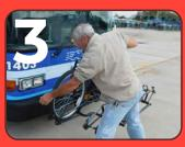
To unload, release support arm and lift bike from the rack. Return rack to the upright position.
