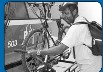
3. To unload, release support arm and lift bike from the rack. Return rack to the upright position.
