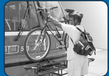
2. Place bike wheels into slots labeled "front" and "rear." Pull out bike support and lift it over front wheel. The spring in the arm will keep your bike secure while the bus is moving.
